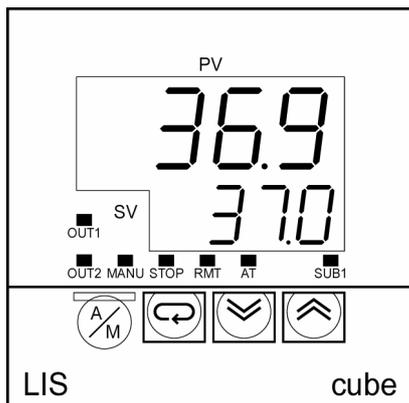
The OUT1 indicator flashes with the control period of the controller. The relative duration of the flash indicates the duty cycle of the output. The other keys and indicators are not used in normal operation mode. Their function is described below.
